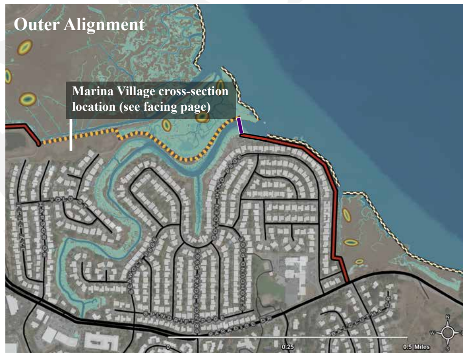
Figure 3.8. Graphic representation of a potential outer alignment and tide gate designed to protect Mariner Cove and Marina Village.
