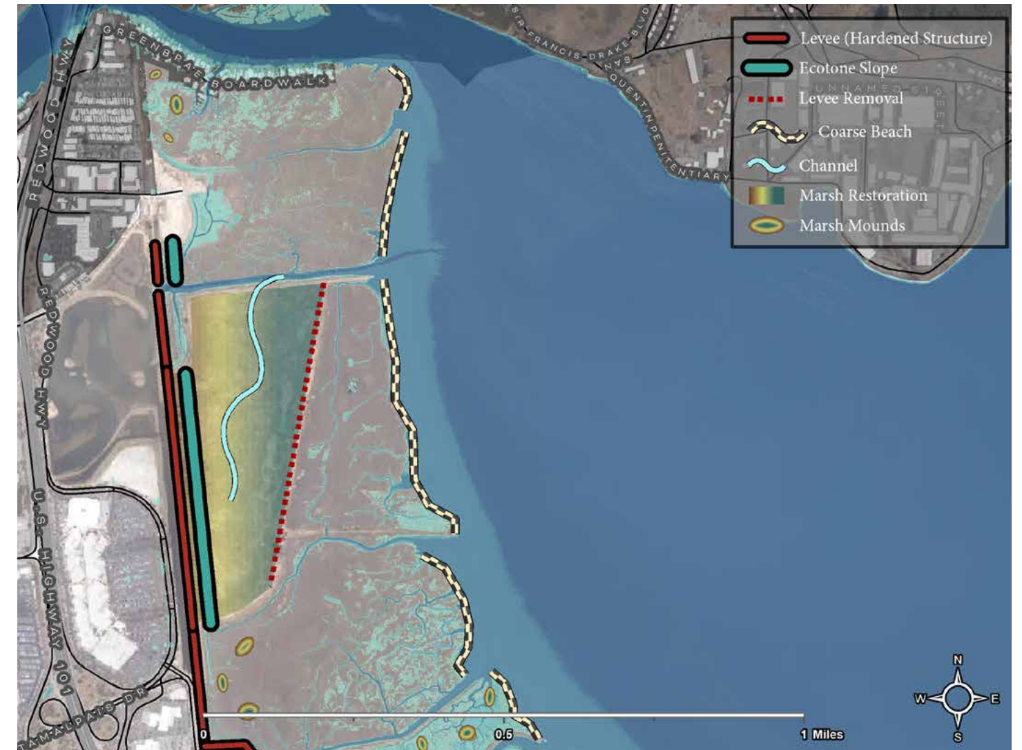
Figure 3.19. Conceptual design for potential restoration and adaptation options at Corte Madera Marsh and the railroad right-of-way.
