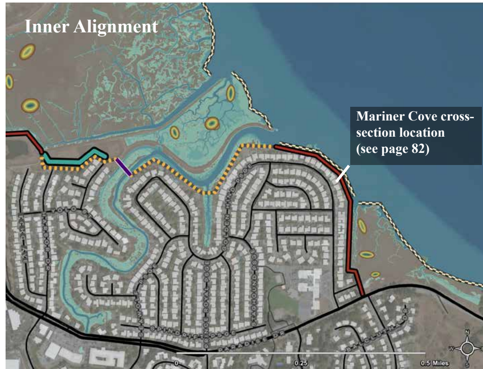
Figure 3.7. Graphic representing a potential inner levee alignment and tide gate designed to protect Mariner Cove and Marina Village.
